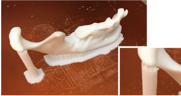
Fig. 2.10 Model of a hemimandible 3D printed using a material extrusion printer. Inset shows the typical striations on the surface of models printed with this technology due to its typically lower layer resolution than other
