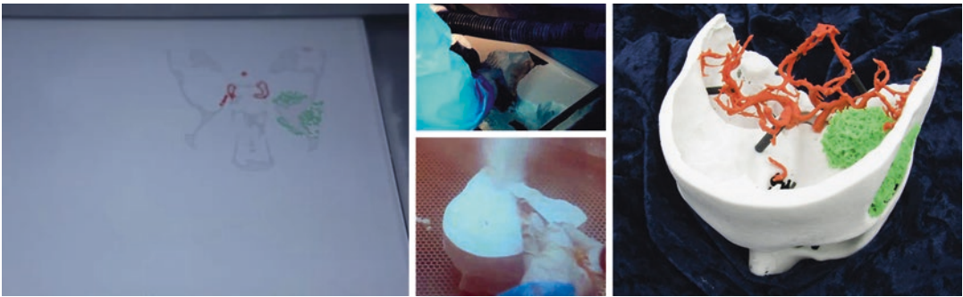
Fig. 2.9 Model of skull printed using a binder jet printer. Powder bed onto which colored binder has been laid is shown mid-print ( left panel ). Once the print is completed, the model is dug out from the powder using a vacuum
