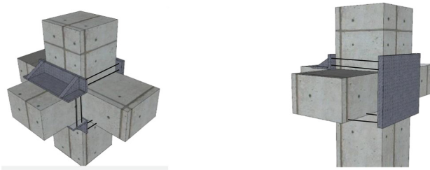
Fig. 8. The exterior beam column joint model retrofitted specimen-2
