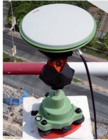
b. GNSS antenna coupled with 360° prism reflector.
