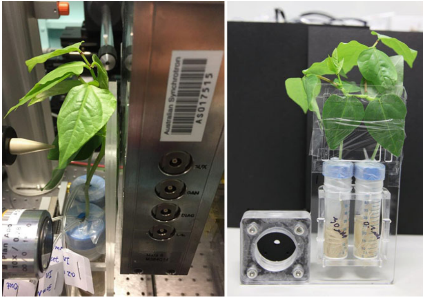
Fig. 8 Live plants (cowpea, Vigna unguiculata ) to be analyzed with the Maia detector system at the XFM beamline of the Australian Synchrotron. The leaves
