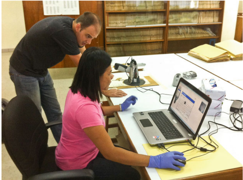
Fig. 2 The typical setup during XRF scanning of herbarium specimens, here conducted at the Forest Research Centre herbarium in Sabah, Malaysia. The herbarium specimen sheet is placed on a titanium metal sheet that serves as a X-ray radiation block, with the portable XRF device fitted with a backscatter shield placed. The XRF device is connected to a computer to read out the acquired data
