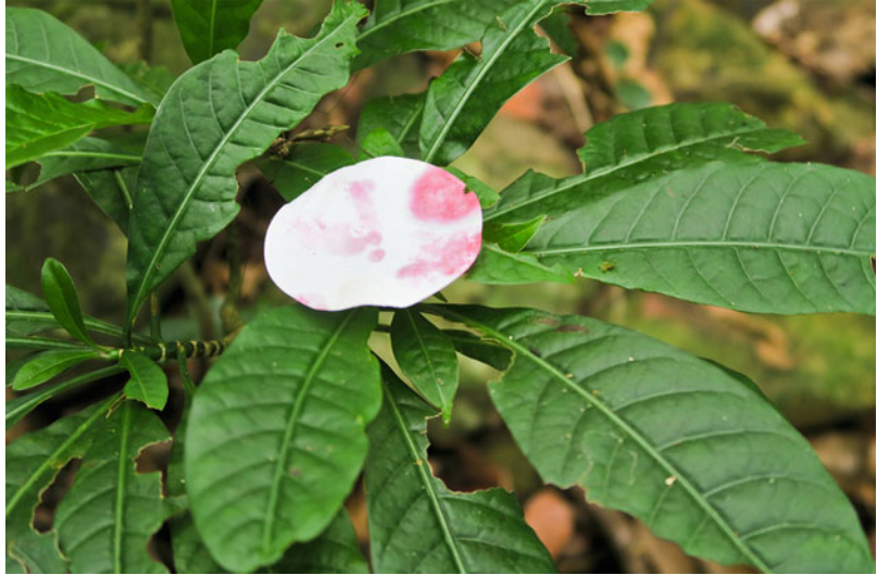
Fig. 1 Field spot test based on the Ni-specific colorimetric reagent dimethylglyoxime demonstrating the reaction with Ni from the fresh leaf of the Ni hyperaccumulator species Psychotria gabriellae (Rubiaceae) in the field in New Caledonia. The test is fast and sensitive and has aided in the identification of numerous Ni hyperaccumulators globally
