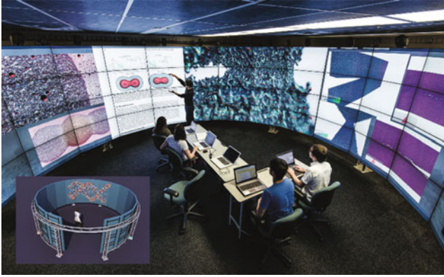
Fig. 18 Students having an immersive meeting in CAVE2. The space can comfortably accommodate up to seven individuals with chairs and tables. CAVE2 can be used to effectively juxtapose 2D, 3D, and abstract data, as well as text documents
