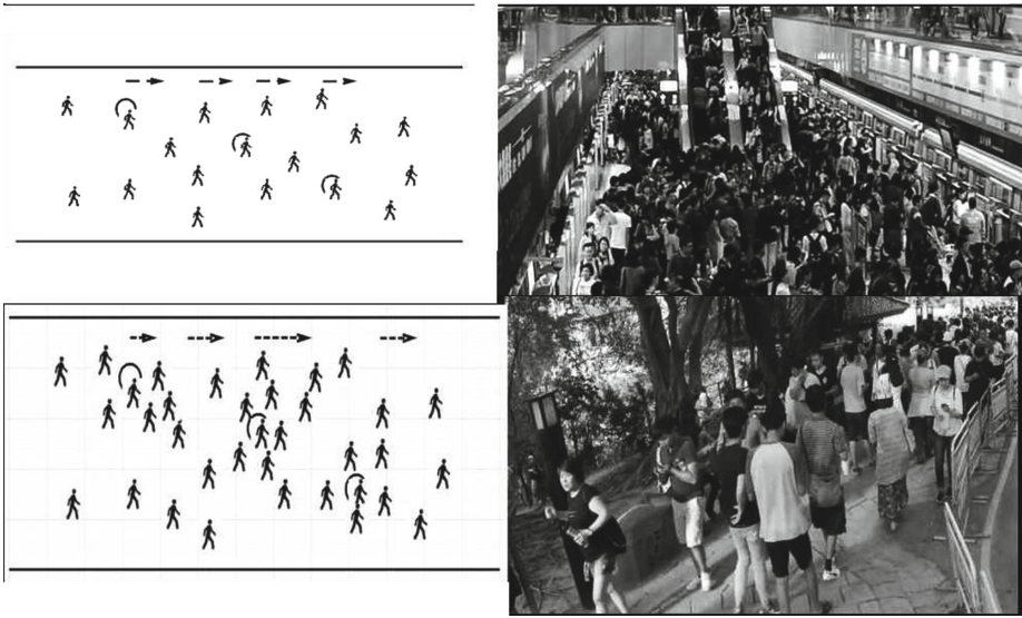
Fig. 1. Relations among speed, density, and tracking devices. Individual tracking devices are shown in circles and the number of devices is far less than the total number of pedestrians.
