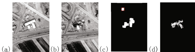
Fig. 4. Comparison between the method and other methods in damage detection. (a) Image before damage; (b) Image after damage; (c) The feature map of the first group is obtained by this algorithm; (d) The feature map of the first group is obtained by literature [10]; (Color figure online)
