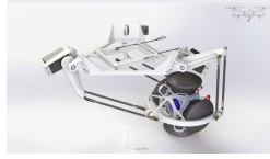
Fig. 1. Sensor deployment and retrieval mechanism
