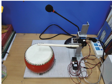
Fig. 1. Robot platform developed for the experiment. The robot platform contains a cylinder drum, a 100 Hz to 16 kHz frequency response hyper cardioid microphone, a panel, a Dynamixel RX-28 servo actuator and its RS485 connector.
