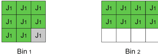
Fig. 3. Illustration of difference in internal fragmentation from job placement
