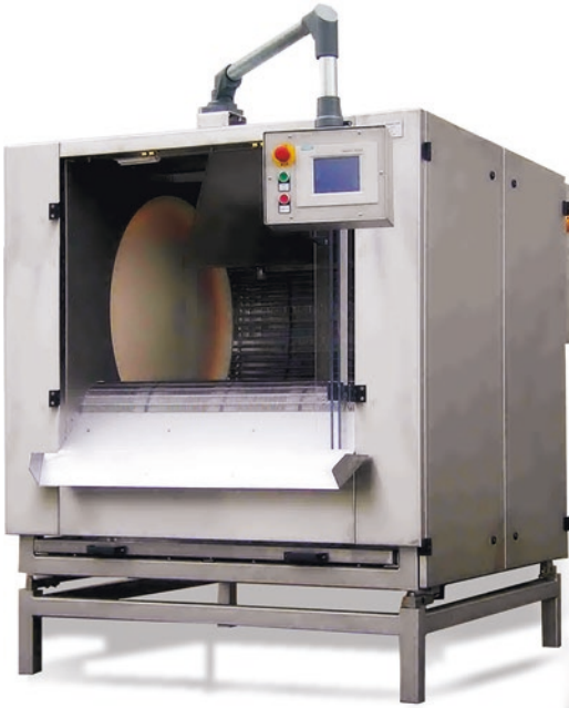
Figure 13.7 Belt coater (Courtesy of Driam)
