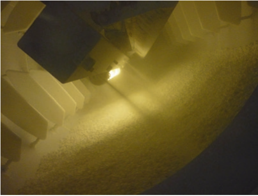
Figure 13.9 Sugar spray system inside drum coater (Courtesy of Dumoulin)
