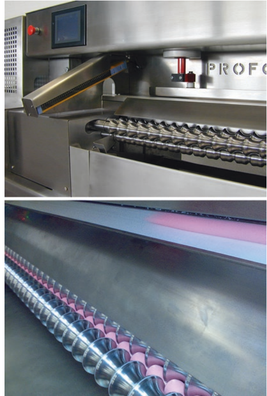
Figure 8.11 Ball roller: top , open with three sets of rollers visible; bottom , balls being formed (Courtesy of Proform)
