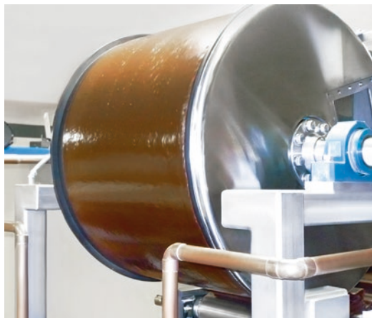
Figure 10.5 Cooling wheel for cooling caramel (Courtesy of R. Hohberger, SPEC Engineering)
