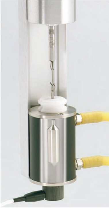
Figure 15.19 Concentric cylinder rotational viscometer used for measuring rheological properties of chocolate (Courtesy of Brookfield)
