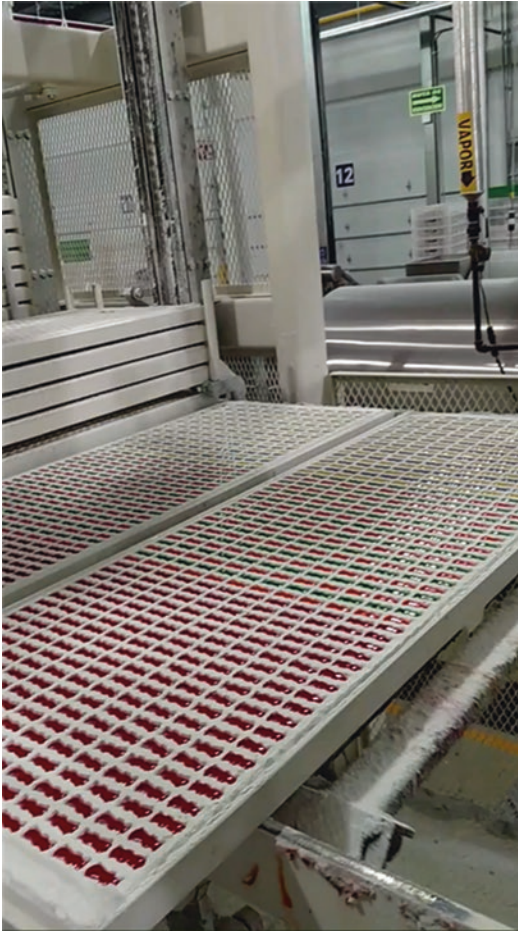
Figure 12.5 Starch tray filled with gummy candies (Courtesy of Fast Track Engineering PTY, Ltd.)
