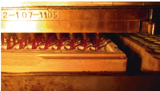
Figure 12.3 Depositing of jelly candy mass into a starch mold (Courtesy of Fast Track Engineering PTY, Ltd.)
