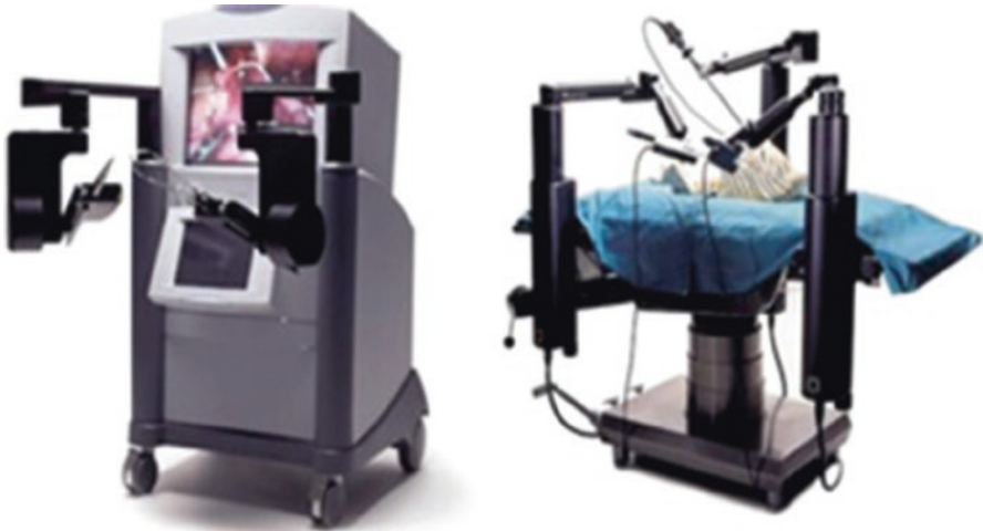
Fig. 20.6 The ZEUS Robotic Surgical System (ZRSS) was a medical robot designed to assist in surgery, originally produced by the American robotics company Computer Motion
