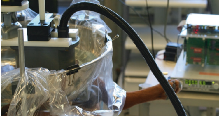
Fig. 23.2 The histotripsy transducer is positioned over the lower abdomen of a canine subject positioned supine. The focal volume of the transducer is co-localized within the prostate. A transectal ultrasound probe is inserted in the rectum to provide imaging of the prostate and bubble cloud during treatment. The power supply and driving electronics are seen in the background
