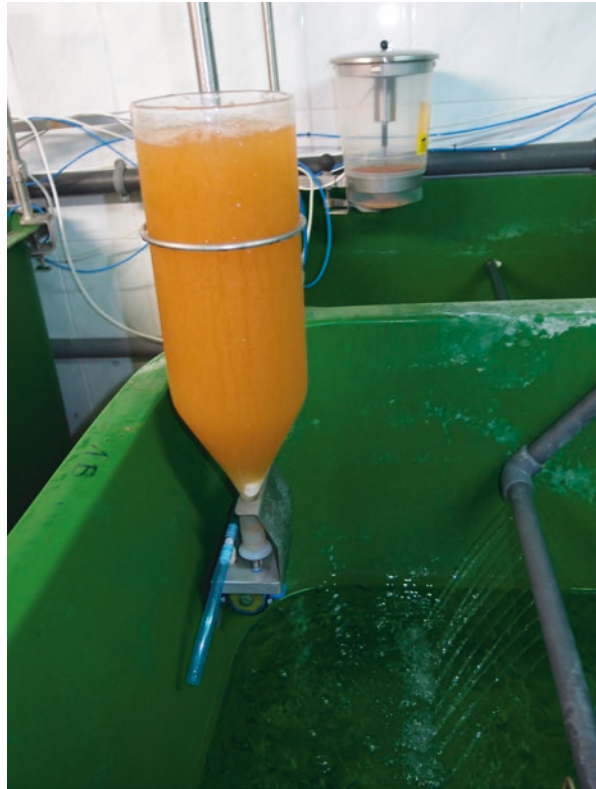
Fig. 30.3 Automatic feeder distributing small granulated feeds (credit L. Kopański)
