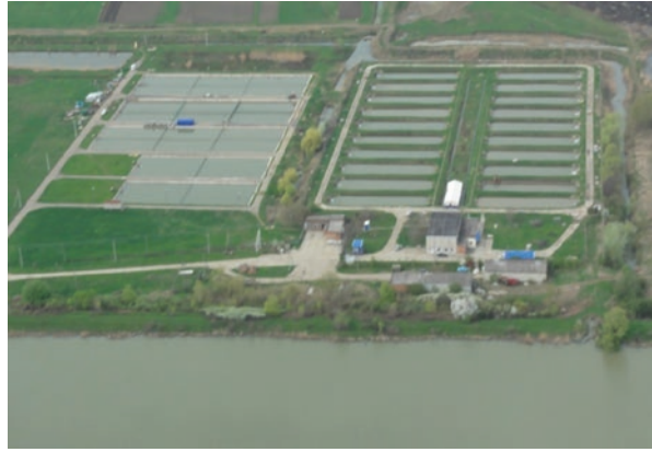
Fig. 38.1 One of the largest sturgeon farms in Russia, the Kuban Sturgeon Farming Institute, Krasnodar region. On the left is a group of concrete pond. On the right side are two series of earth raceways (credit M Chebanov)
