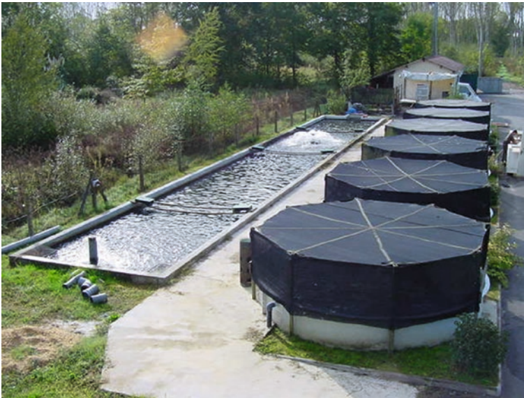
Fig. 38.7 Small raceway separated into three parts and equipped with an aerator (left side of the photo). Small shadowed circular tanks are for holding juvenile sturgeon. Prunier Manufacture sturgeon farm, South West of France (credit P. Williot)
