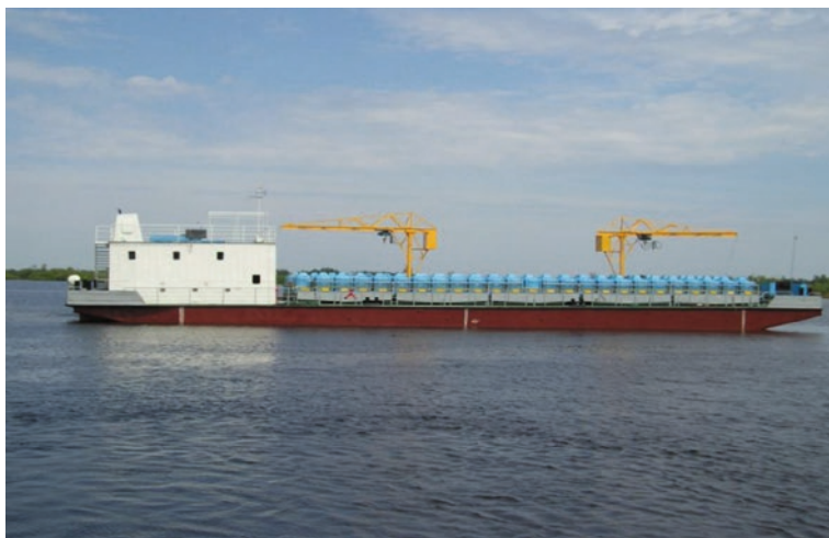
Fig. 37.4 Nonself-propelled experimental fish vessel for fry transportation (created in Gosrybcenter 2007)
