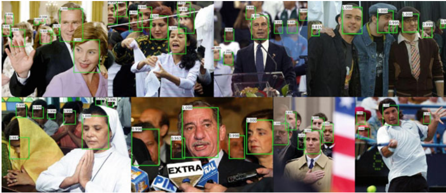
Fig. 3.11 Some examples of face detection results using our proposed CMS-RCNN method on FDDB database [20]
