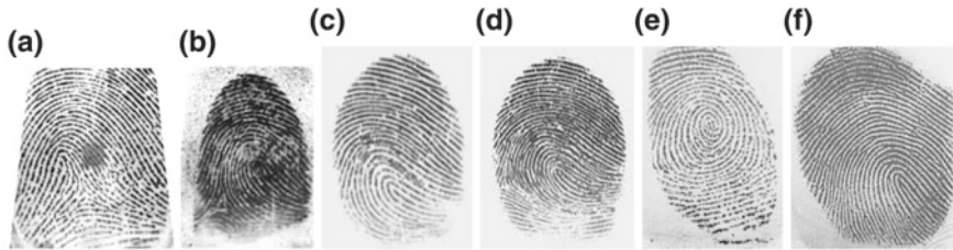
Fig. 12.2 Examples of fake acquisitions from the LivDet 2011 competition (cooperative). From Biometrika a Latex, b Silicone, from Digital c Latex, d Gelatine, from Sagem e Silicone, f Play-doh
