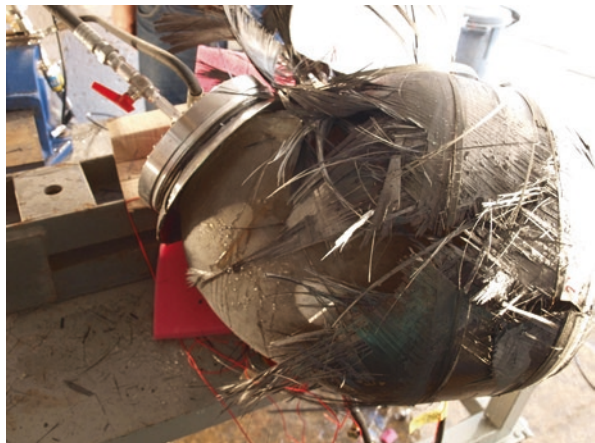
Fig. 23 Burst of vessel #5. AFT boss is being pulled out by the rubber bladder
