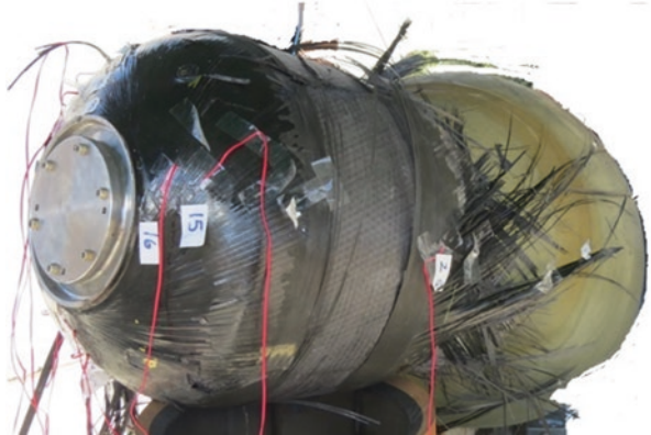
Fig. 28 Burst of vessel #3
