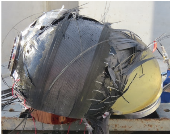
Fig. 29 Burst of vessel #4. AFT boss is being pulled out by the rubber bladder
