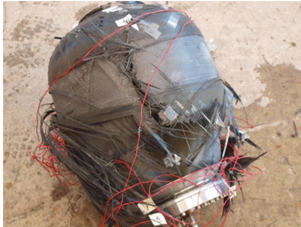
Fig. 20 Tensile strains in the hoop layers, vessel #1 during burst test
