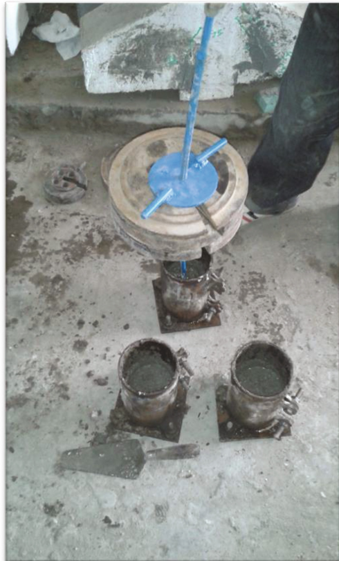
Plate 2. Compaction of Cubes and Cylinders Specimens.
