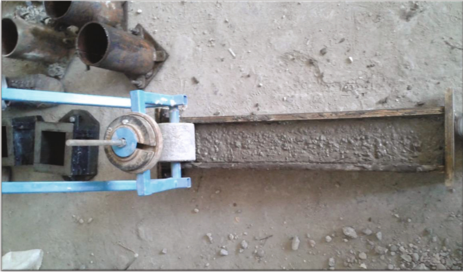
Plate 1. Roller Compacted Concrete.
