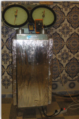
Fig. 2. Thermal enclosure design: temperature control and stabilization accessories
