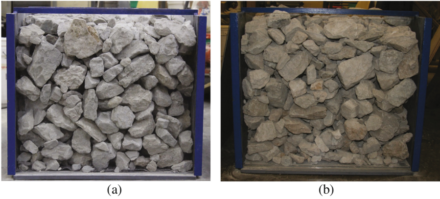
Fig. 3. Cross sections of the compacted large aggregates in (a) One lift and (b) Two lifts
