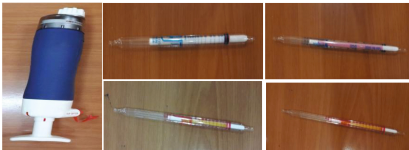
Fig. 13. Drager equipment and emissions tubes.
