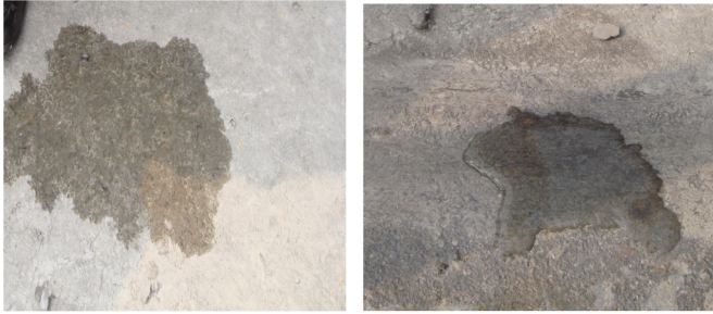
Fig. 4. Water pouring tests: (a) water dispersed on a not-well-formed membrane; (b) water beads on a well-formed membrane
