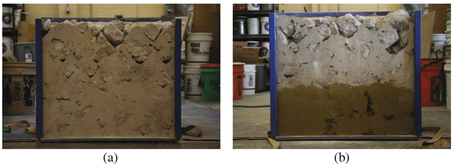
Fig. 7. Cross sections of the compacted large aggregates with 25% of wet QB by dry weight of CS02 on top of (a) Rigid steel bottom (b) Soft compacted subgrade soil
