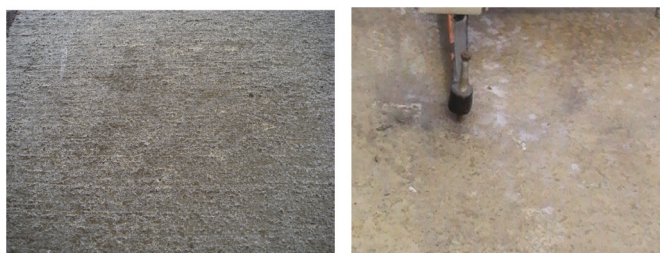
Fig. 3. Surface conditions of formed membrane of EWCA: (a) powder present on surface if membrane is not well-formed; (b) dense surface of a well-formed membrane
