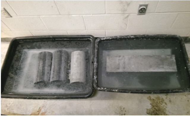
Fig. 2. Water bath curing at room temperature
