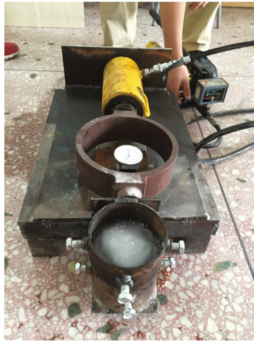
Fig. 6. Tests for interlayer shear bond stress and composite friction coefficient.
