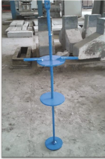
Plate 5. Cube and Cylinder Specimens Compactor.
