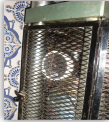
Heating plate mounted on the metal grid
