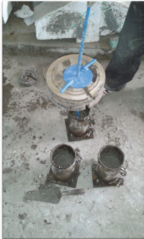
Plate 2. Compaction of Cubes and Cylinders Specimens.
