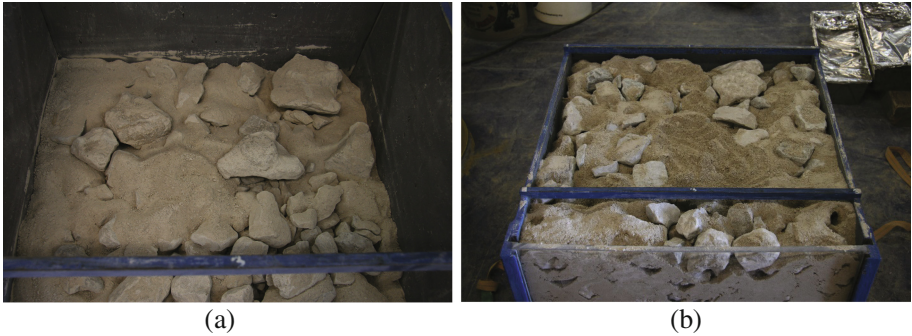
Fig. 6. Top views of the surface of the compacted large aggregates with (a) 40% dry QB and (b) 30% QB with 2.5% moisture content showing roughly similar quantities remaining on the surface
