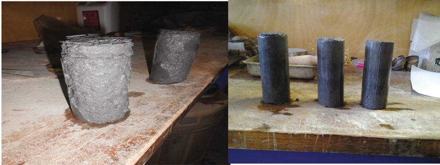
Fig. 3. (a) Typical ash containing 2% cement (b) Typical 8% cement stabilized ash
