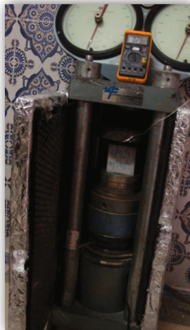
Fig. 2. Thermal enclosure design: temperature control and stabilization accessories
