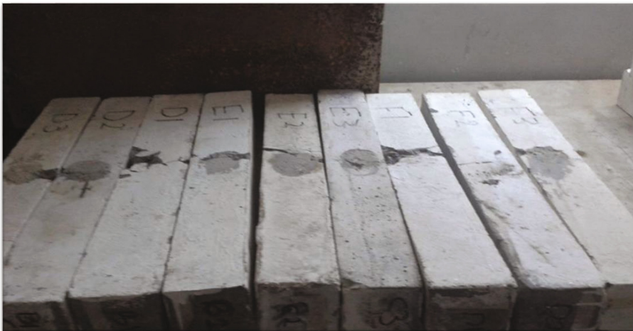
Plate 6. Failed Beam Specimens Roller Compacted SFRC under Impact Load Test.
