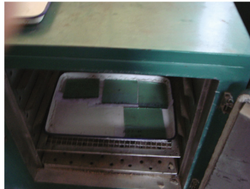
Fig. 2. Tests for membrane forming and thermal endurance of EWCA on glass plates
