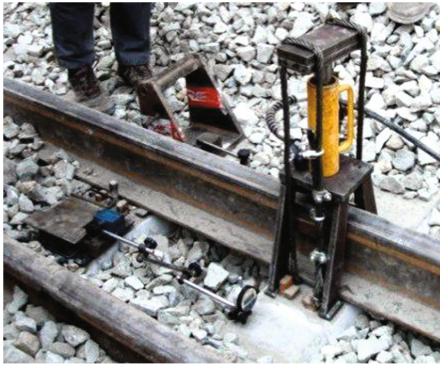
Fig. 6. Test of ballast bed's vertical stiffness
