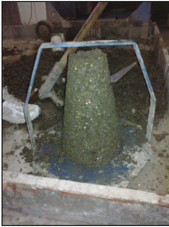
(a) Slump test
