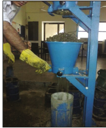
(b) Compaction factor test
