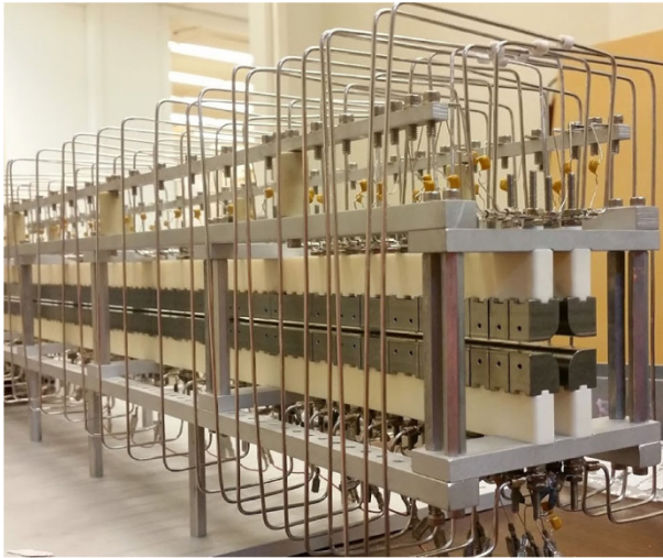
Fig. 3 The RFQ structure with in-vacuum RF and DC circuitry during test-assembly
