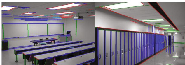
Fig. 4. Lines extracted in orthogonal directions of indoor scenes
