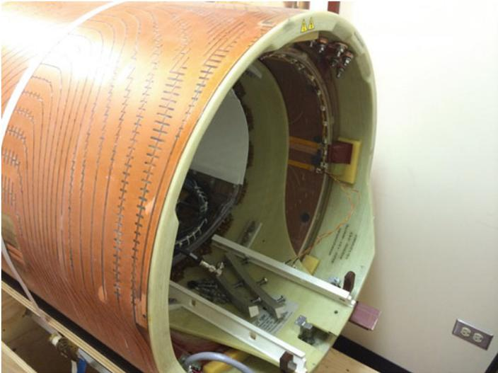
**Fig. 9.3** Gradient system of an MRI system with  $x$ -,  $y$ -, and  $z$ -gradient coils embedded in epoxy. The gradient coils are used to localize the MR signal from a specific location in the human body
