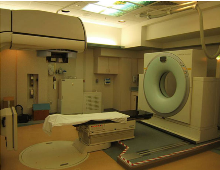
Fig. 5.4 (a) A Siemens CT-on-rails system at the Medical College of Wisconsin (Courtesy of Medical College of Wisconsin, Milwaukee, WI)
