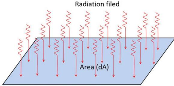
$$\psi = \left( \frac{d(NE)}{dA} \right) = \left( \frac{dN}{dA} \right) E = \phi E \quad (2.3)$$
