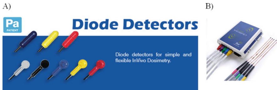
Fig. 13.10 (a) Diode detector from Sun Nuclear Corporation, (b) MOSFET detector from Best Medical LLC
