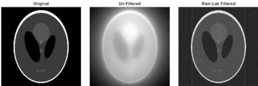
Fig. 6.20 Comparison of reconstructed image without and with Ram-Lak filter
