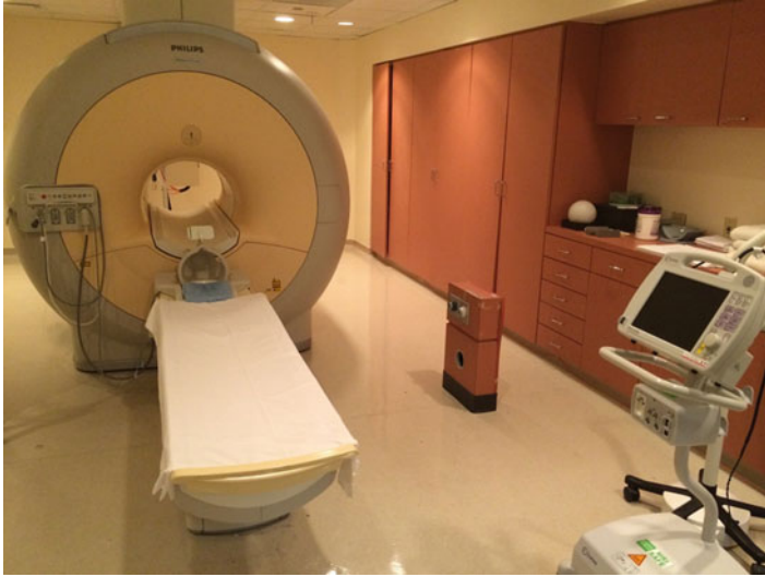
Fig. 9.1 Clinical MRI system with the patient table in the front that can be moved inside the bore of the magnet
