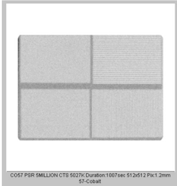
Fig. 11.7 Extrinsic resolution image of Co-57 flood source on parallel hole collimator. A Co-57 sheet source was on top of a four-quadrant resolution phantom positioned on top of the parallel hole collimator loaded onto the detector head (images were from Nuclear Medicine Service, Virginia Commonwealth University Hospital System, Richmond, Virginia)
