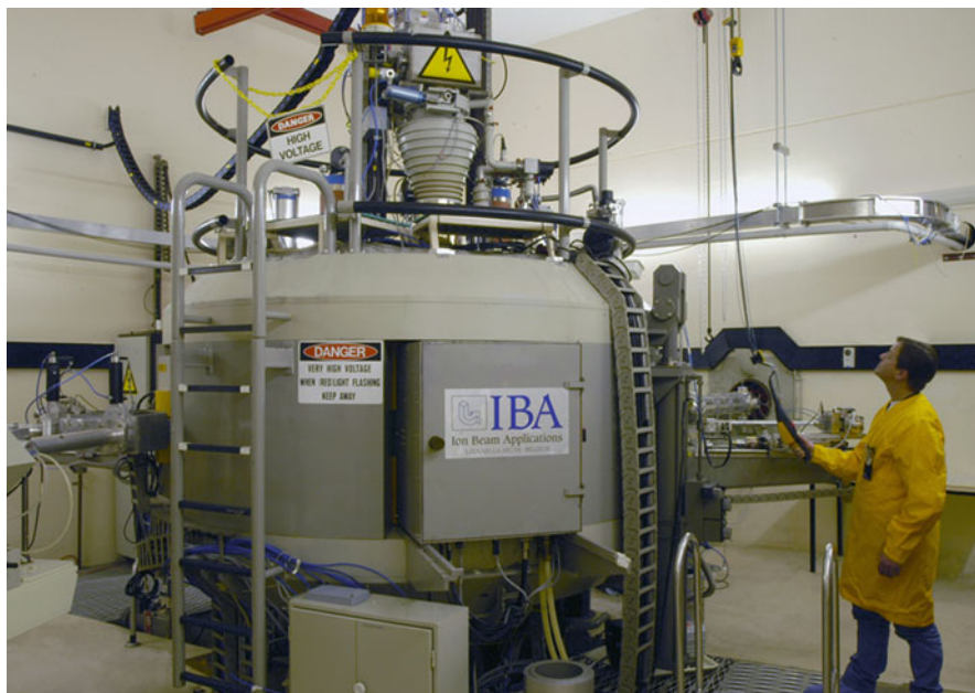
Fig. 11.1 Cyclotron used for radioisotopes production
