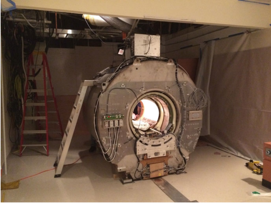
Fig. 9.2 Superconducting magnet of a clinical MRI system after the removal of the covers and the patient table
