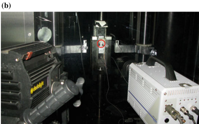
Fig. 1 Two experimental configurations using one high-speed camera (FASTCAM APX RS, Photron, Japan) and powerful lighting (Dedolight 400D, Dedotec, Germany). The monitored sample is encircled in red. a Taken from [24], b Courtesy of N. Swiergiel (Airbus Group Innovations)
