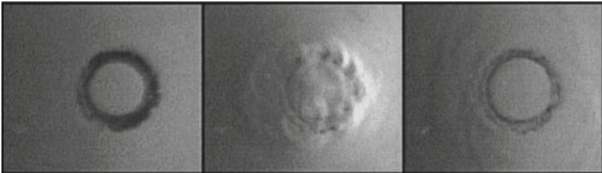
Fig. 11 Shock waves from a laser-induced bubble collapsing near a flat, solid wall in bottom view. Image converter camera, one million frames per second. Frame width 4.2 mm. See also Philipp and Lauterborn [10]
