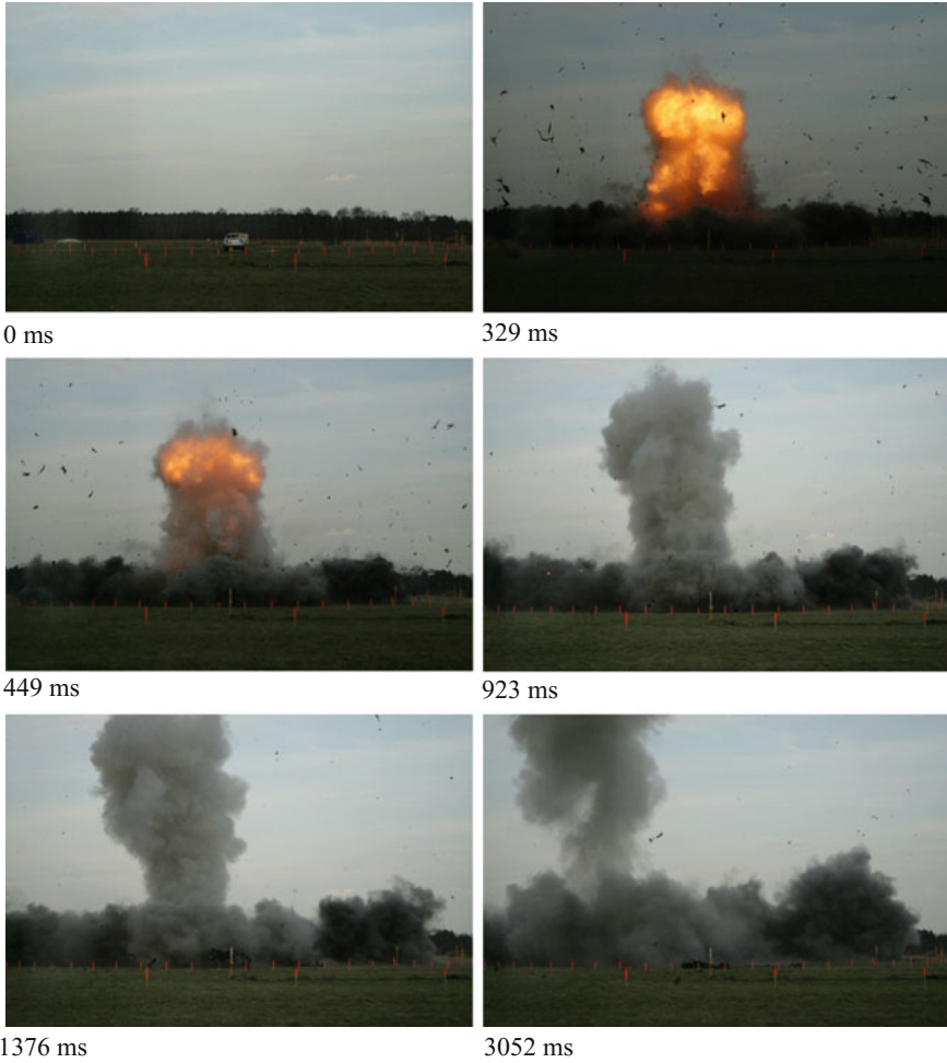
Fig. 6 Sequence of video stills from VBIED-test conducted by WTD 52 and WTD 91. Times below indicate the time span from initiation. Images used by kind permission of WTD 52
