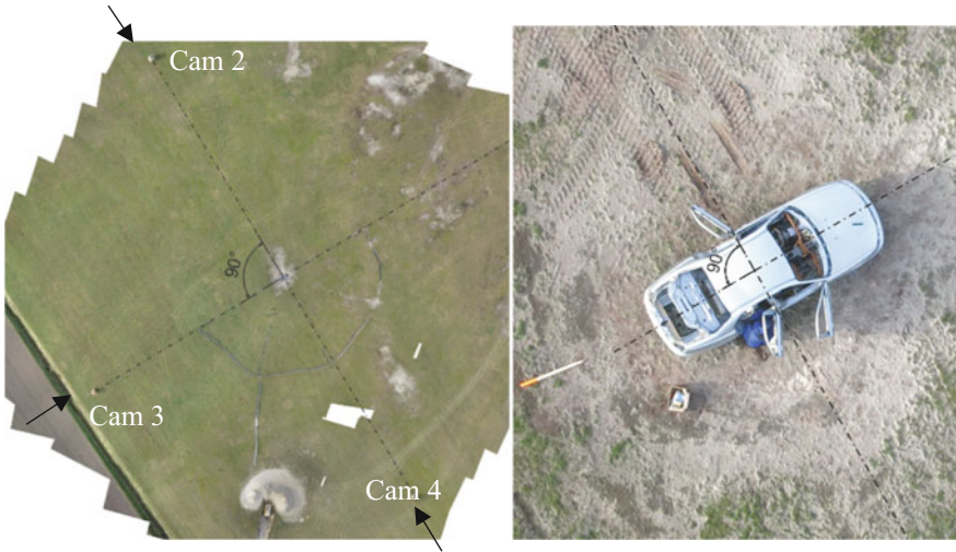
Fig. 4 Left , aerial view of experimental set-up. Explosion site in the center . Right , close-up of explosion site. Cameras perpendicular to each other, camera 1 beyond picture boundaries
