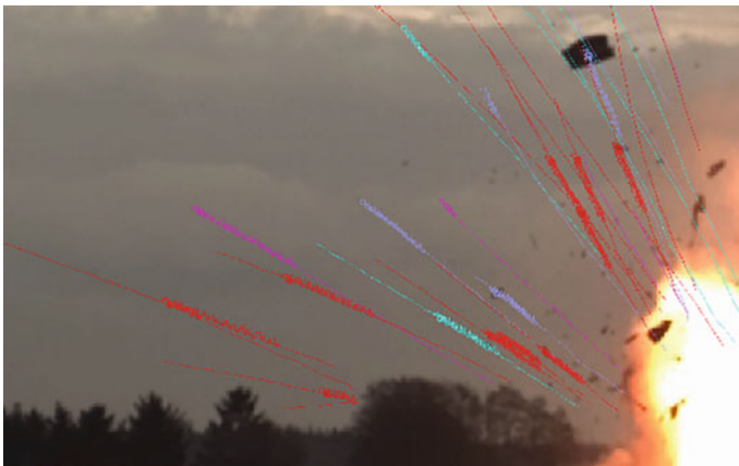
Fig. 5 Screen shot from tracking software. The fragments are distinguished by their masses, indicated by line color and symbol along the respective trajectory
