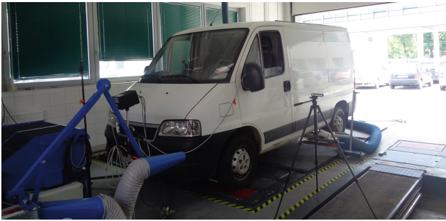
Fig. 4. Dyno recording. OBD acquisition shown, and the audio recorder (on the tripod)
