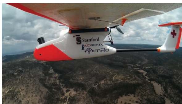
Fig. 11.2 Fixed-wing drone. Picture taken from the tip of the wing of a fixed-wing drone, during an aircraft test on stress, battery life, and carrying capacity. This unit is equipped with video cameras that transmit video to the remote pilot, so they can see where it is flying (first-person view, FPV) and at the same time sends the telemetry of the aircraft
