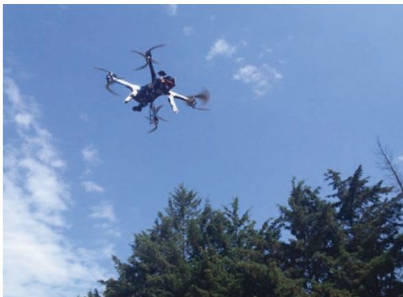
Fig. 11.5 Multi-rotor drone. This image was taken during the search for a missing person in a canyon in Mexico. This 8-motor multi-rotor drone incorporates a video camera that transmits to the operator. However, the range of operation is short. This is an ideal platform when takeoff space is limited or when there is not enough space for the operator to move around
