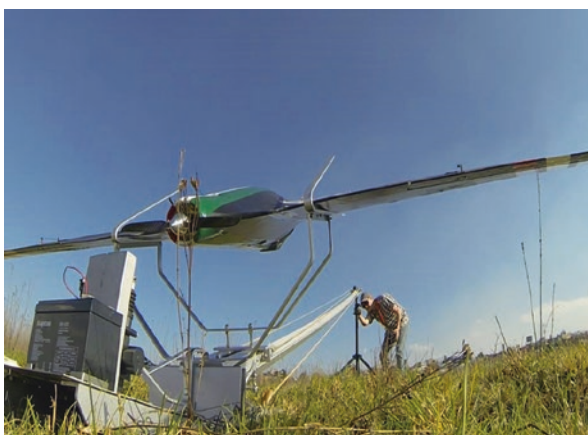
Fig. 11.4 Delta fixed-wing drone. This is a delta fixed-wing drone of 2-m wingspan. Due to its heavy weight, it is released by means of a catapult. This is one of the prototypes used to transport medical supplies to rural communities. Its approximate flight time is 45 min and cruising speed is 70 km/h
