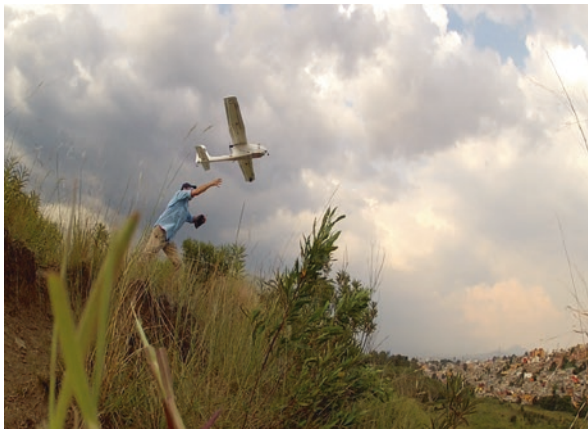
Fig. 11.3 Manual launch of a fixed-wing drone. Manual launch practice of a fixed-wing drone built by Aidronix. Manual launch of a drone can be very complicated as human error can compromise the aircraft. Additionally, the operator is at very close proximity to the propeller, which can be dangerous. In larger units this technique is impractical due to the total weight of the aircraft
