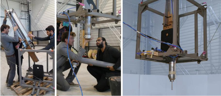
**Fig. 3.** Assembly of Pylos extruder on Cogiro.
