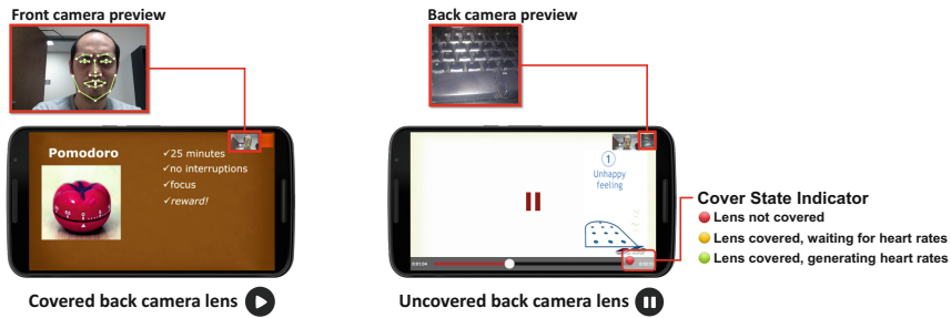
Fig. 1. AttentiveLearner 2 uses both the front and the back cameras as feedback channels: back camera for PPG sensing and front camera for facial expression analysis (FEA).
