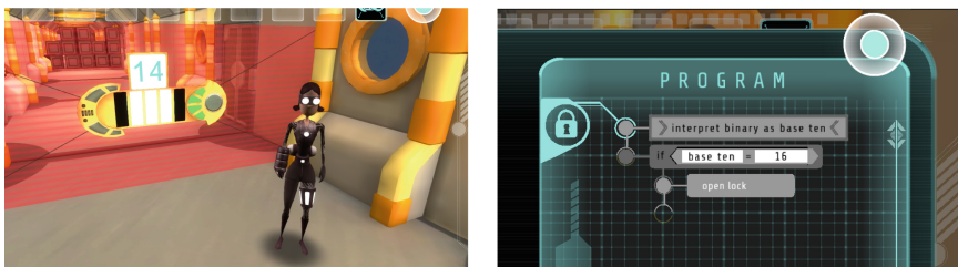
Fig. 2. (Left) A binary lock device that students must unlock. The white tiles indicate the bits are 1, whereas black tiles denote 0. The current binary number is 01110 and the corresponding base-ten number, 14, is displayed on the device as immediate feedback. (Right) The visual programming interface displaying the binary lock's program.
