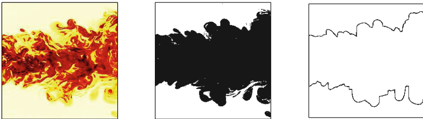
(a) Original image (b) Binarization and contour tracing (c) Contour smoothing
