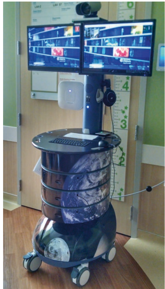
Fig. 14.2 A telehealth cart, which includes a web camera, monitors, and keyboard for documentation, for use in an ambulatory clinic. Photo courtesy of the Telehealth Center at Cincinnati Children's Hospital Medical Center
