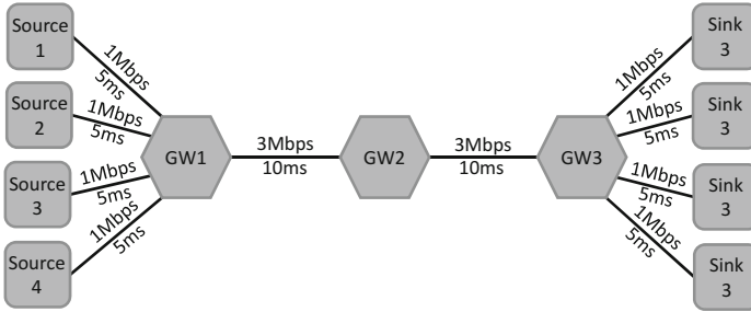
Fig. 5. The network topology
