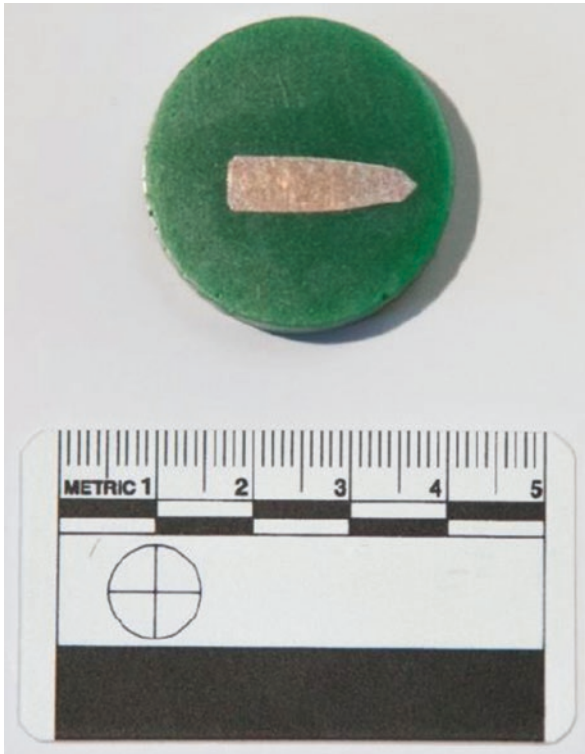
Fig. 2.11 Frangible Bullet shown in cross section
