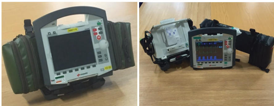
Fig. 28.2 Corpuls [3] monitor, patient box and defibrillator/pacer. Combined together with the associated cables and consumables in side pouches ( left ). Broken down into the three component parts ( right )
