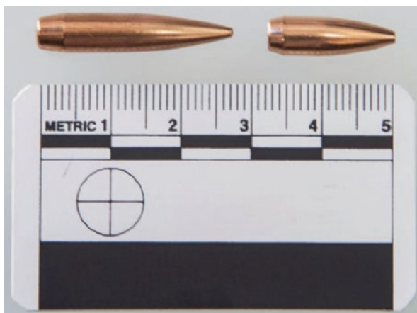
Fig. 2.4 Photograph showing two 0.223" bullets: ( Left ) an 80 Grain Sierra and ( Right ) a 52 grain Speer (HP Boat Tail Match)
