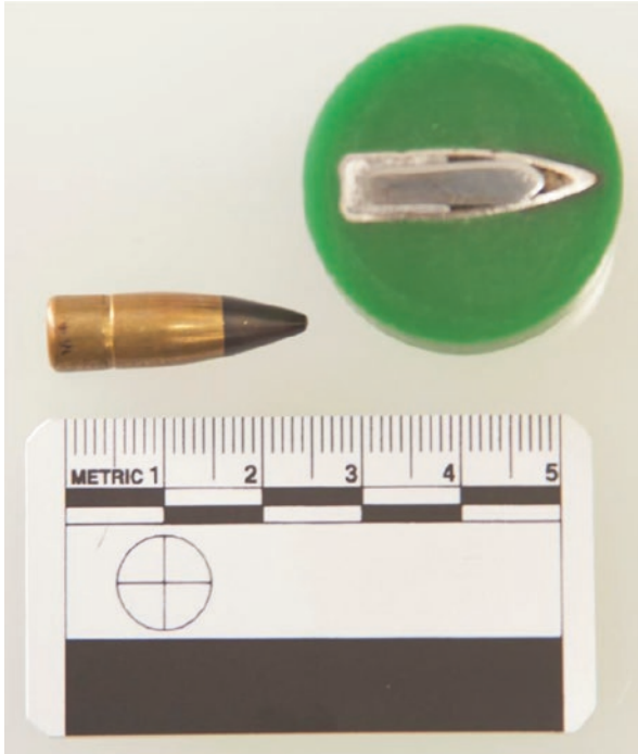
Fig. 2.8 Photograph showing a Full Metal Jacket Armour Piercing Bullet with a hardened penetrator core visible in cross-section
