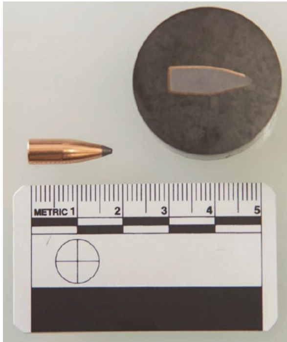
Fig. 2.10 Photograph showing a Soft Point Bullet and in cross section
