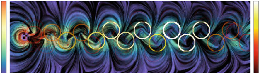
Fig. 9 Output of Algorithm 1 for the pattern from Fig. 8 in the strain tensor field of the von Kármán vortex street laid over the tensor LIC of the major eigenvector. The color in the LIC corresponds to the Frobenius norm of the strain tensor, the color of the circles to the similarity
