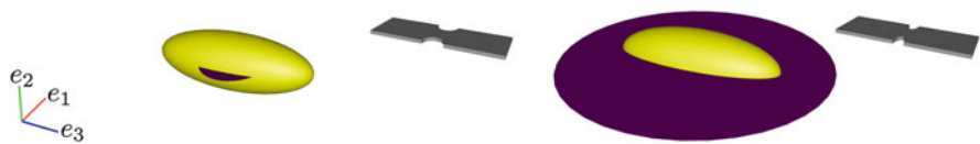
Fig. 9 The purple ellipsoid shows the overall change of the stress tensor in all spatial directions, the yellow ellipsoid visualizes the stress tensor. The left image corresponds to the less curved tensile bar, the right image to the stronger curved tensile bar
