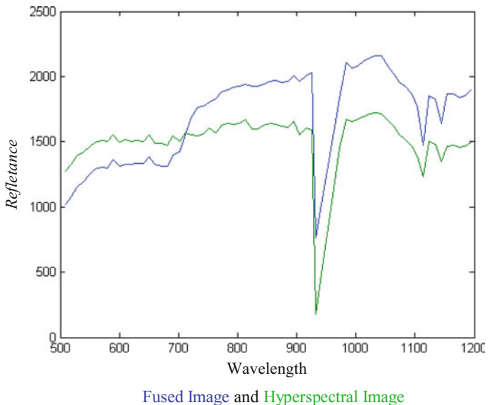
Fig. 13 Spectral profile of beach (soil) pixels of fused and hyperspectral image
