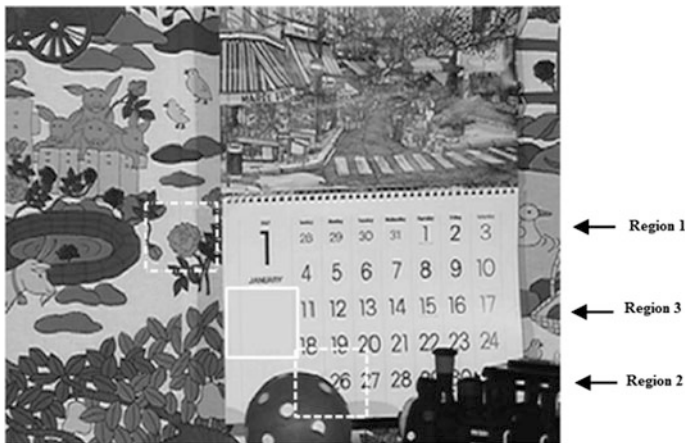
Fig. 8 Region 1 (R1) has a textured area with translational motion, Region 2 (R2) shows a textured area with independent object motion, and Region 3 (R3) contains a flat area with translational motion
