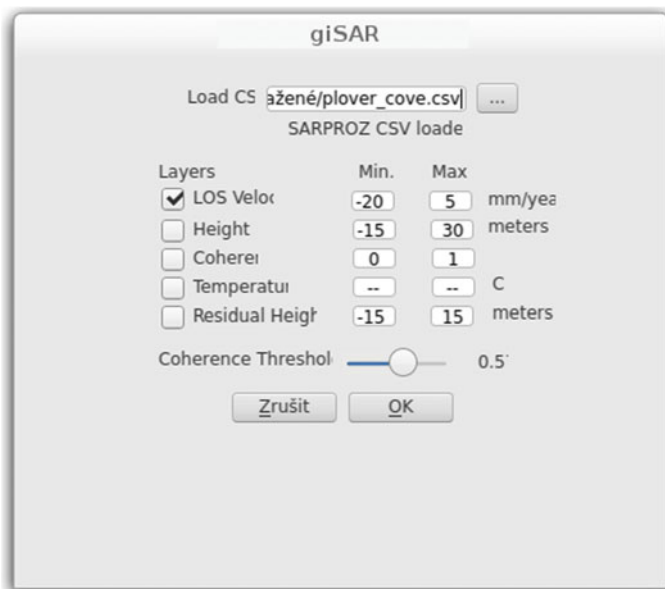
Fig. 2 Basic window of Quantum GIS: giSAR toolbox offering preliminary functionality of importing InSAR-based CSV file as GIS layers
