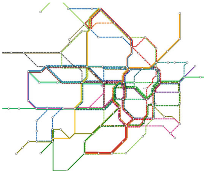
Fig. 4 Final result after applying the GA for octilinear path schematization in Castellón bus network
