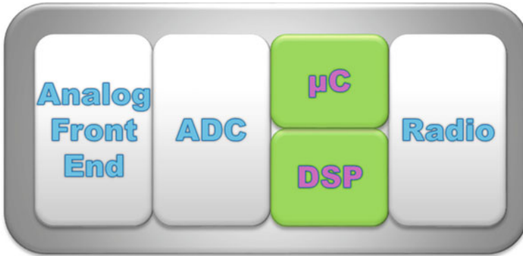
Fig. 7.1 General block diagram for a wearable healthcare device
