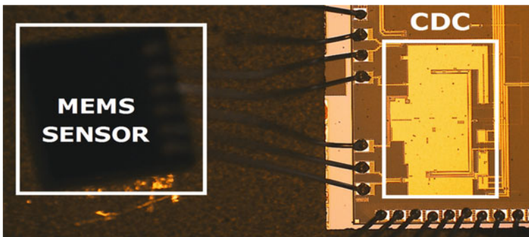
Fig. 11.9 Die photo of the MEMS sensor and the CDC in the same package
