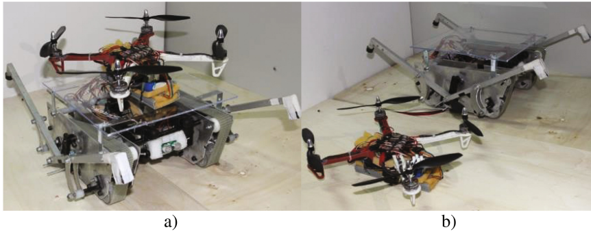
Fig. 1. The proposed ground/aerial robot composed by the two modules: (a) in a combined operation mode; (b) the ground and aerial modules for an in parallel operation.
