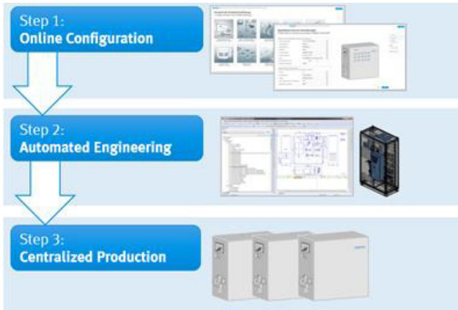
Fig. 5. Control cabinet: from online configuration to production
