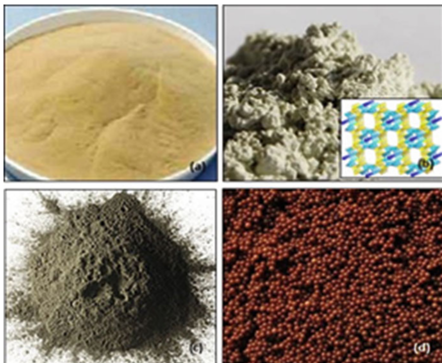
Fig. 2.6 (a) Palygorskite, (b) zeolite with structure as inset, (c) fly ash, and (d) polymer resin as adsorbents
