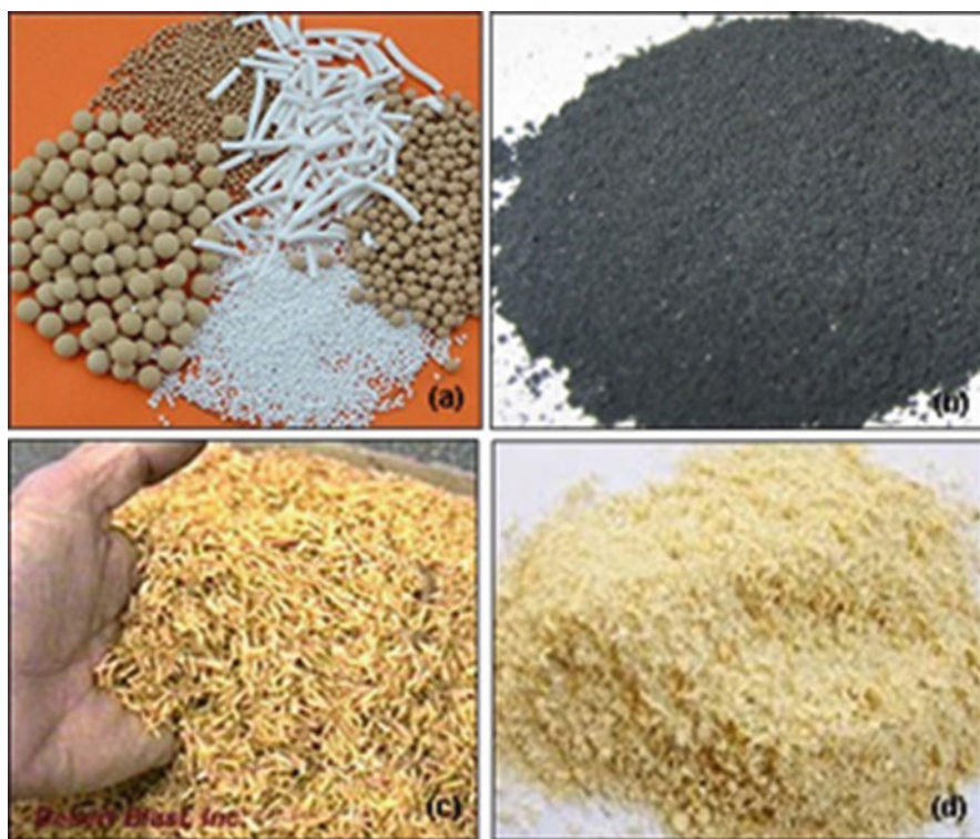
Fig. 2.5 Adsorbents used for removal of metal from water: (a) activated alumina, (b) activated carbon, (c) rice hull, and (d) corncob
