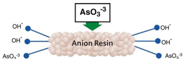
Fig. 2.3 Removal of \text{As}^{+3} from water using anion-exchange resin
