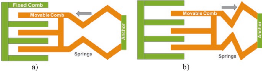
Fig. 12.9 Comb electrostatic MEMS actuator: (a) actuator in on , (b) actuator in off
