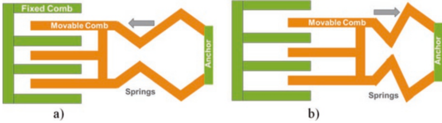
Fig. 12.9 Comb electrostatic MEMS actuator: (a) actuator in on , (b) actuator in off
