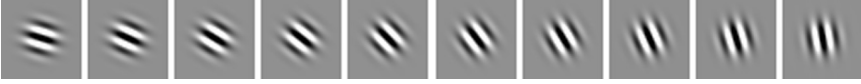
Fig. 3. Wavelet filter bank. The figure shows 10 selected orientated wavelets ranging from 17^\circ to 80^\circ in increments of 7^\circ .
