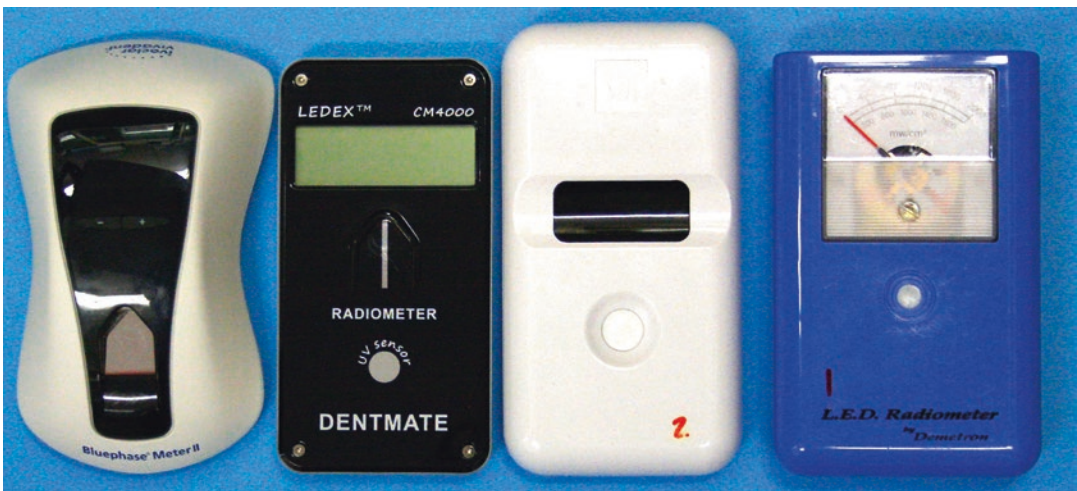
Fig. 4.9 Examples of four commercial dental radiometers. The Bluephase Meter II on the left has a large entrance aperture and currently is the only dental radiometer that is able to measure all the power from a 13-mm diameter light tip
