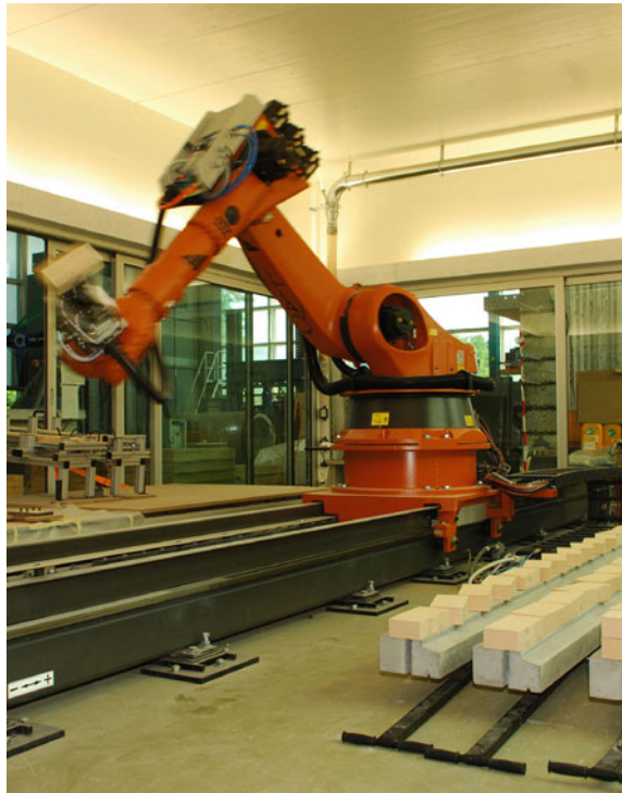
Fig. 6 © Gramazio Kohler Research, ETH Zurich pre-fabrication steps of the modular wall of the leading Facade Wineyard Gantenbein at ETH Zurich. (Left) Used with permission
