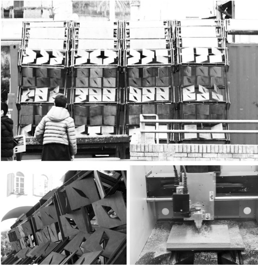
Fig. 5 Folding foyer. Details of the continuous roof and CNC machinery production process
