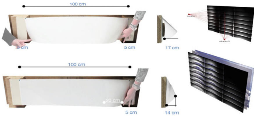
Fig. 1 Left Maximum bending deformation of the physical prototype. 8 cm inwards results in 17 cm of displacement at mid-span. Right System: simulated bending behaviour of all modules of the system. Bending deformation varies according to users position in space
