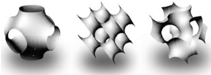
Fig. 4 From left: P Surface \cos(x) + \cos(y) + \cos(z) = 0 ; D Surface \sin(x) \sin(y) \sin(z) + \sin(x)\cos(y) \cos(z) + \cos(x) \sin(y) \cos(z) + \cos(x) \cos(y) \sin(z) = 0 ; Gyroid \cos(x) \sin(y) + \cos(y) \sin(z) + \cos(z) \sin(x) = 0
