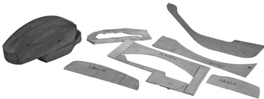
Fig. 1 Wooden model with dime of the Grillo phone, Marco Zanuso and Richard Sapper for Siemens, 1965 photography: Federico Pollini—Archive Giovanni Sacchi
