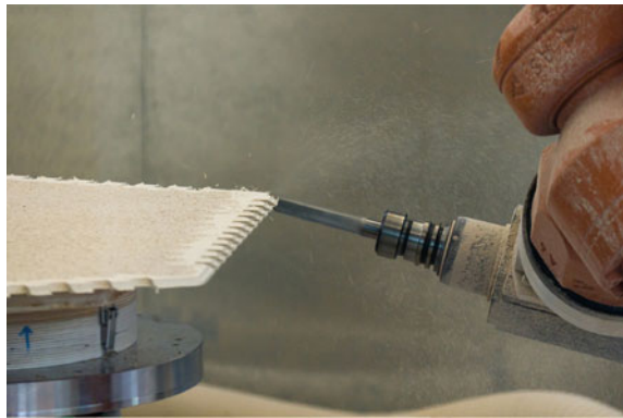
Fig. 3 © ICD/ITKE Research Pavilion 2011 cutting finger joints ( top right )
