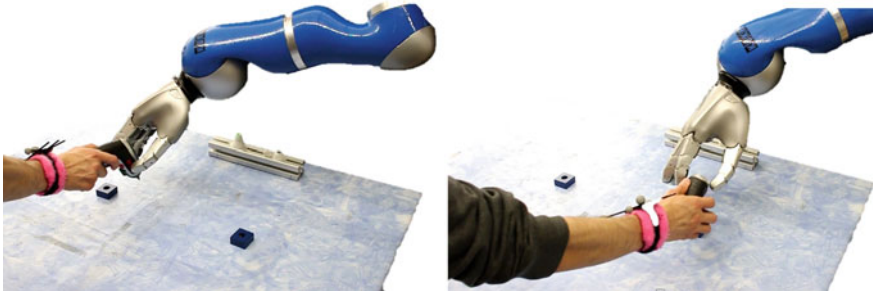
Fig. 6 Handover and return of a screwdriver at different positions, obtained by conditioning the Interaction ProMP on the positions of the wrist marker
